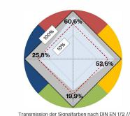
transmission of signal colours acc. to EN 172
